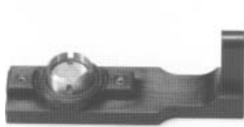
Fig. 4.8: Desiccant covered with spacer plate with notches properly aligned.
