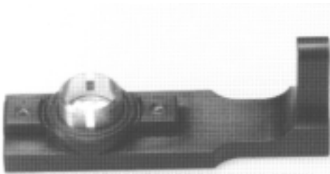
Fig. 4.7: Cup with desiccant inserted.
