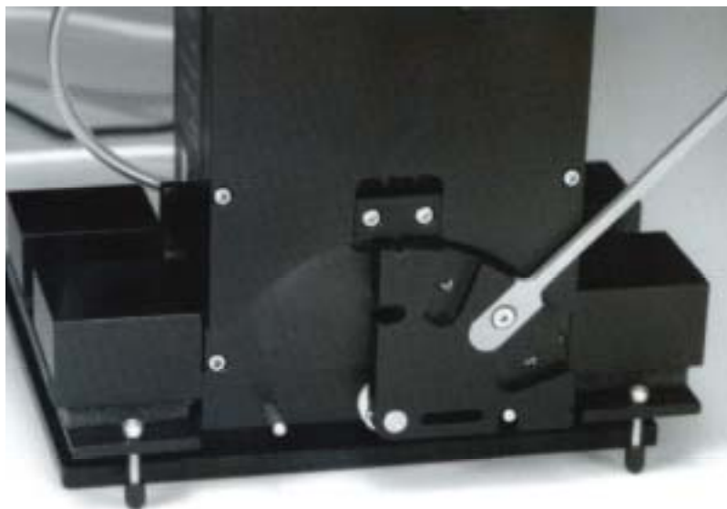
Fig. 3.5a: Extra support screws can be used at the rear of the detector. Note the three slots that the lever can mate into thus positioning the lever to rotate over a range suitable for different FTIR sample compartments.
