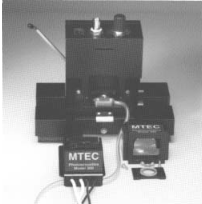
Fig. 6.4: Disassembled unit ready for window replacement.
