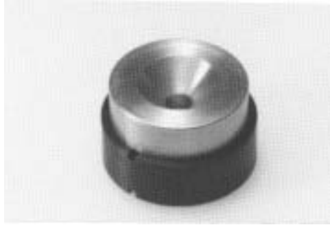
Fig. 4.6: Sample loading funnel and cup fixture.
