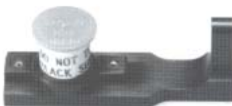
Fig. 4.11: MTEC Carbon black reference. Keep capped when not in use.
