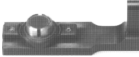
Fig. 3.2: Sample cup with infrared sensing liquid crystals in place.
