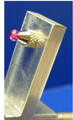
Lapper Arm with protective cap and Ruby Ball Joint exposed. This ball should be protected from shock and abrasion
