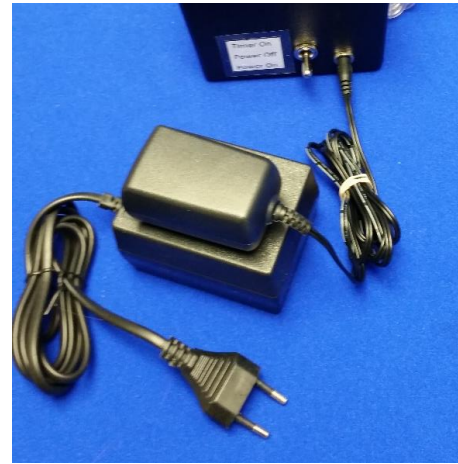
220 V Operation with 220 V to 110 V Converter
