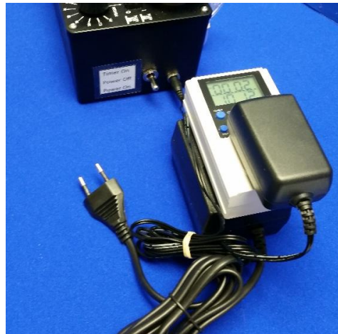
220 V Operation with External Timer (Timer Plugs Directly for 110 V)
