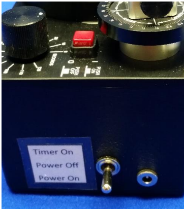
Lapper Power Switch
